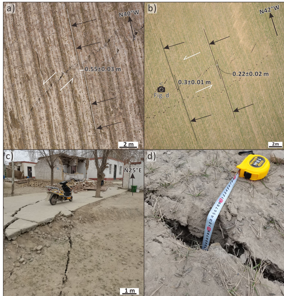
Figure 5. UAV images and photographs of surface rupture in segment (a). (a) The left-lateral displacement is 0.55 m. (b) Left-lateral displacement is 0.24–0.29 m. (c) Severe damage and collapse occurred as the surface ruptured through the house. (d) The depth of surface rupture in section a is ~0.6 m.
