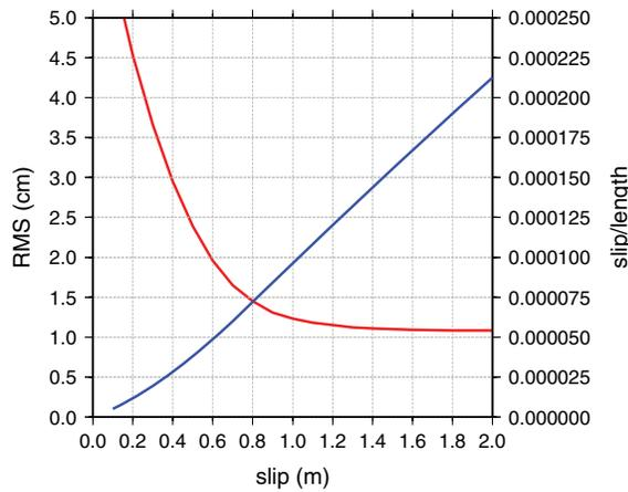
**Figure 5.** Rms misfit (red line) versus magnitude of slip fixed in solving for the Damxung fault geometry. Improvement in fitting the interferogram data becomes insignificant for choices of uniform slip above  $\sim 1$  m, with slip-to-length ratios (blue line) also increasing.
