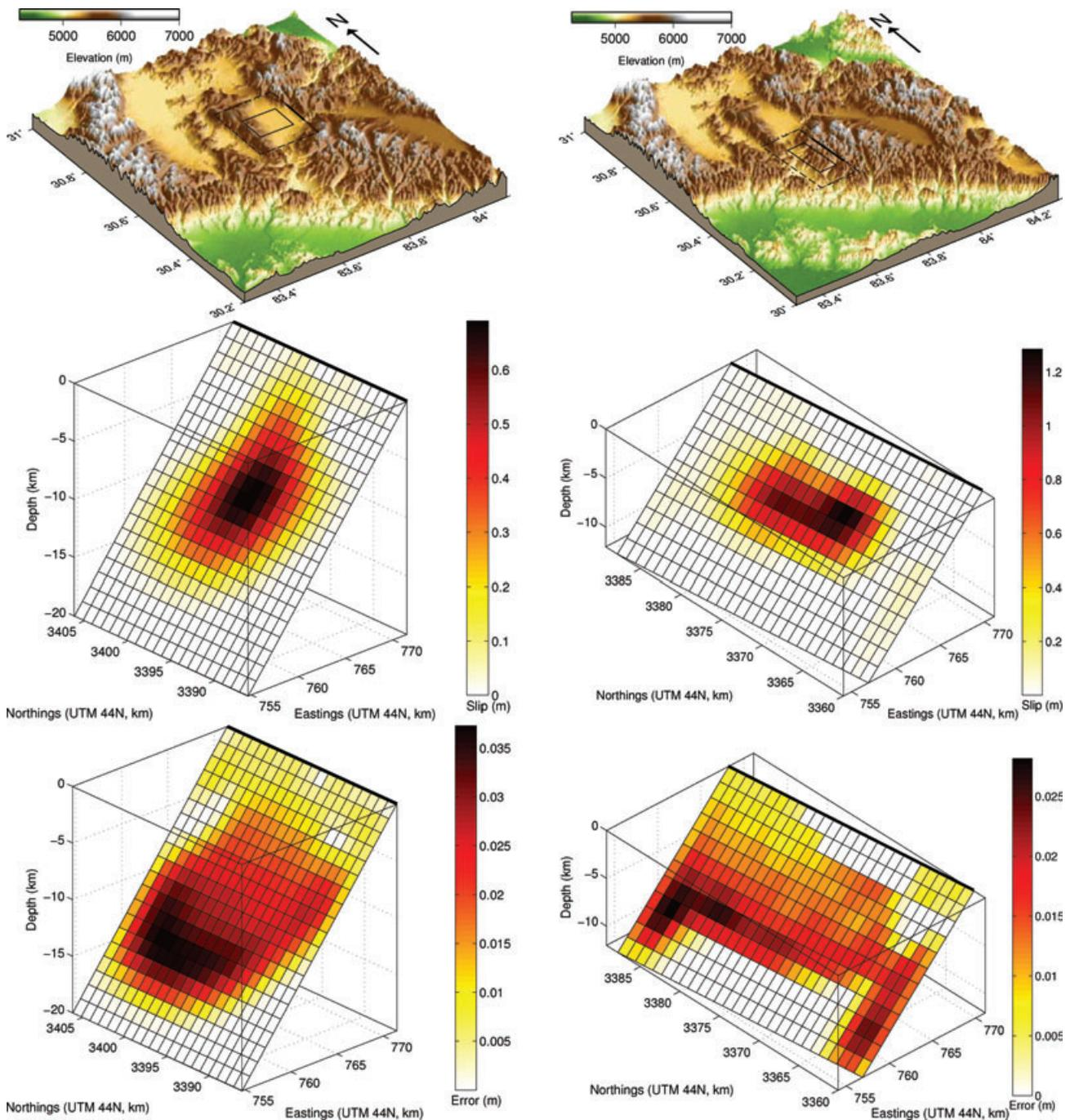
**Figure A2.** Left-hand panel: Zhongba 2004 earthquake slip distribution with fixed rake based upon the fault orientation from uniform slip modelling. Right-hand panel: Zhongba 2005 earthquake slip distribution with fixed rake based upon the fault orientation from uniform slip modelling. Caption as for Fig. 9.
