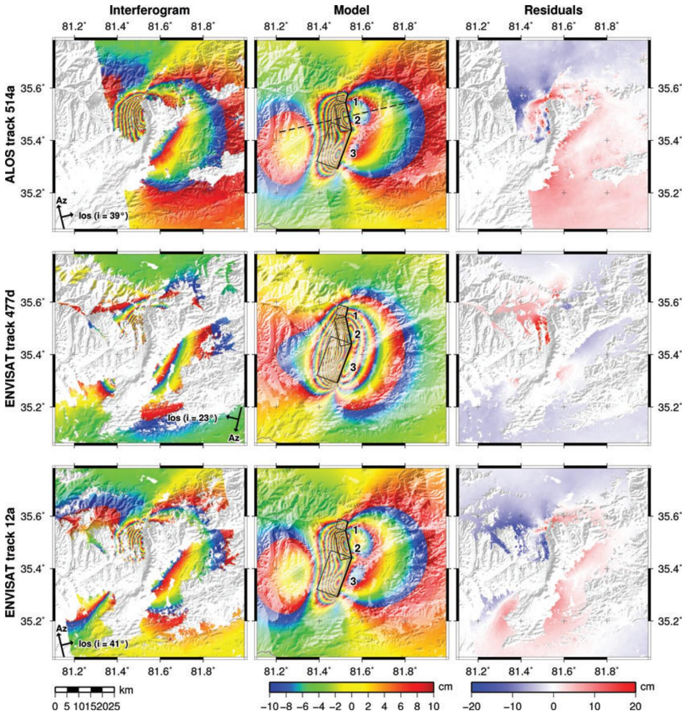
**Figure 13.** Yutian earthquake interferograms for distributed slip with fixed rake models and residuals. Interferograms for the five other tracks used in the modelling, but not shown here, are given in the on-line supporting information. Symbols as for Fig. 4.
