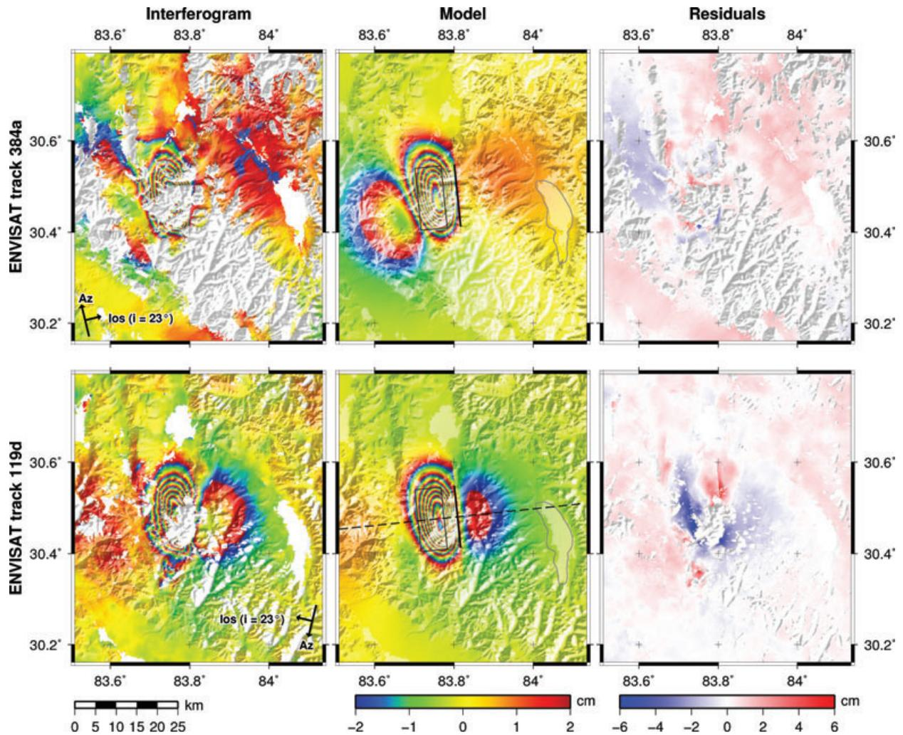
**Figure A3.** Zhongba 2005 earthquake interferograms for distributed slip modelling with fixed rake. The interferogram for the other track used in the modelling but not shown here is given in the on-line supporting information. Details as for Fig. 4.
