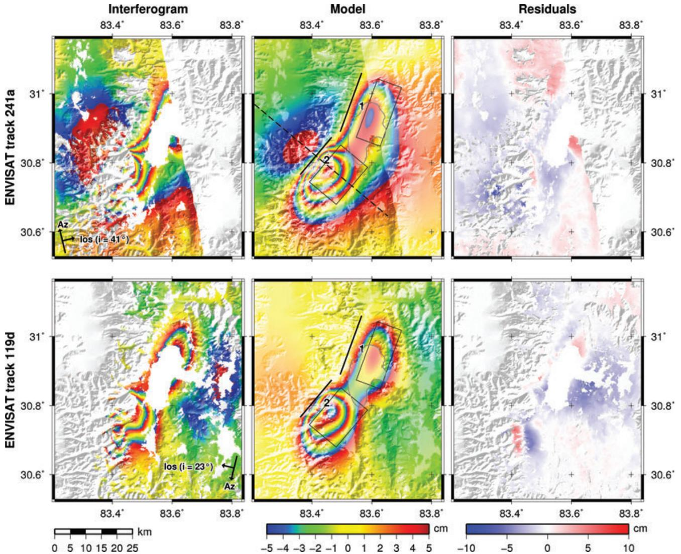
**Figure 16.** Zhongba earthquake interferograms for distributed slip modelling with a fixed rake. Interferograms for the two other tracks used in the modelling, but not shown here, are given in the on-line supporting information. Details as for Fig. 4.
